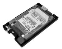
**Step 6** Put the top cover on by holding it in near vertical position and sliding the two metal clips inside the two small slots on the rear of the bottom cover.
